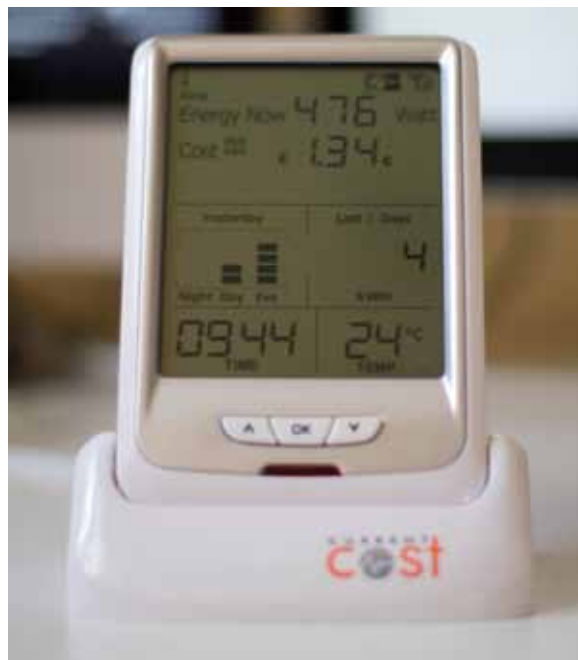
Smart grids can incorporate smart meters and in-home energy monitors, allowing users to better manage their electricity use. Source: flickr/TomRaftery
